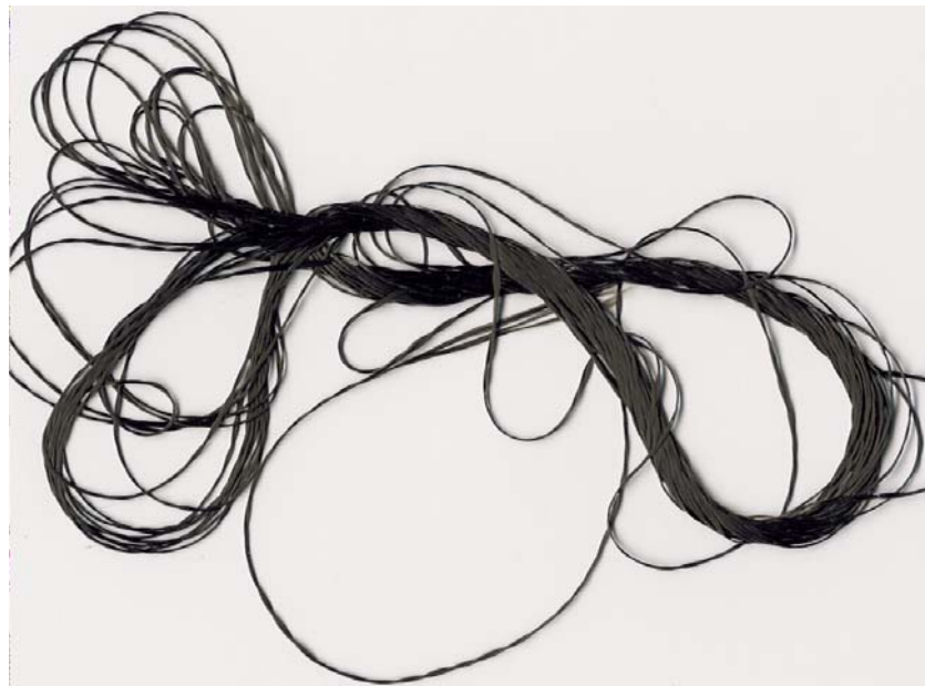
Basalt yarn after forming, twisting and plying 5
