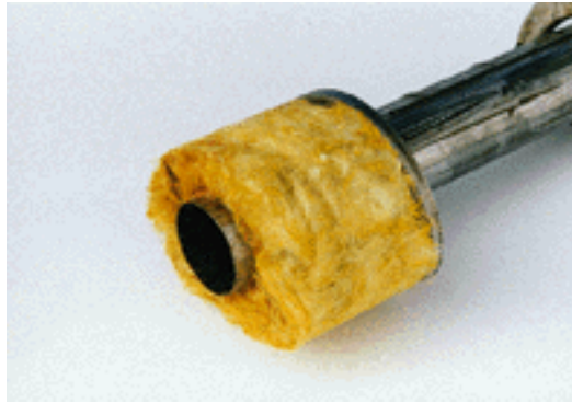
Truck Muffler formed from needed insulation 12
